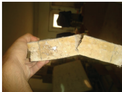
Figure 7. Date Palm Supported Adobe Bricks Failing Flexurally and Demoulding
