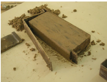
Figure 7. Date Palm Supported Adobe Bricks Failing Flexurally and Demoulding
