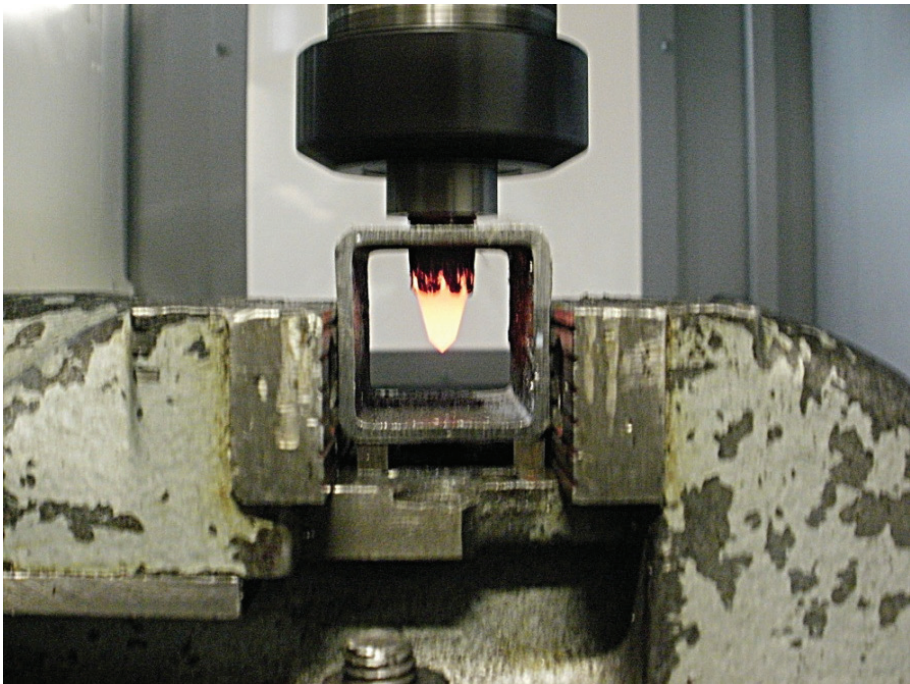
Figure 4. Friction Drilling Application to Welded Square (Doğru, 2010)
