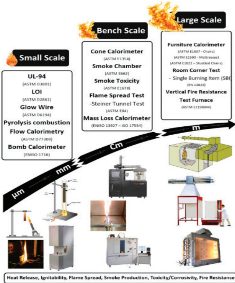
Figure 10. Various Test Methods and Setups Associated with Flame Retardants in Polymer Materials (Vahabi et al., 2021a)
