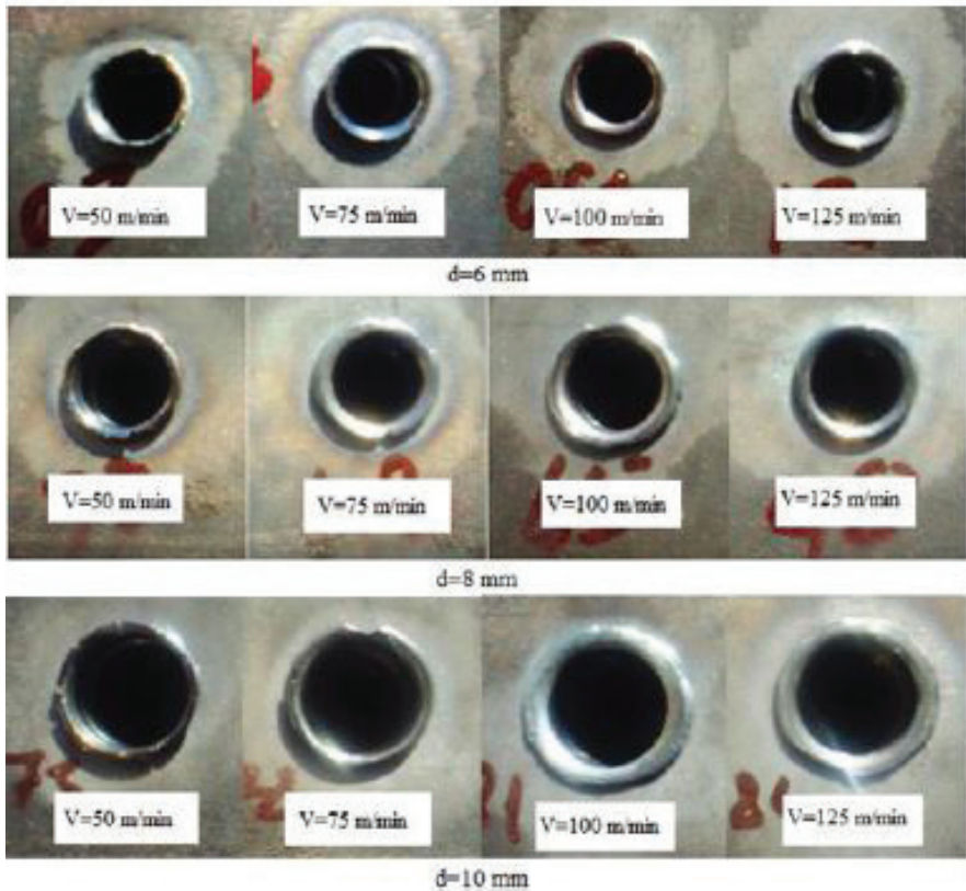
Figure 14. Effects of Different Drilling Speeds on Bushing Geometries at \alpha=30^\circ Tip Angle and f=225 mm/min Feed Speed (Özler and Dođru 2013)
