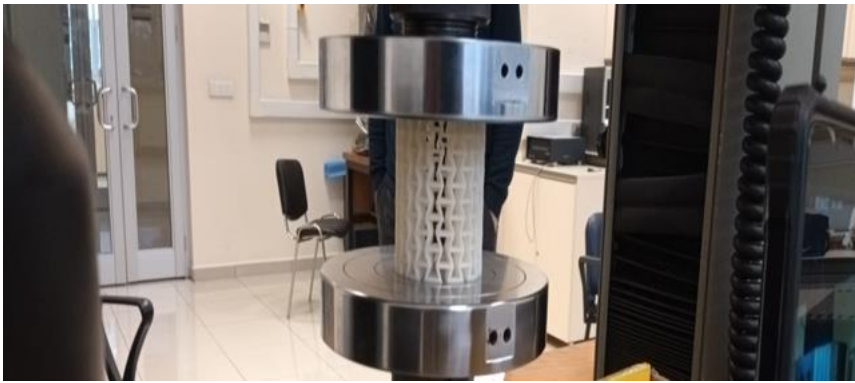
Figure 22. Image of the Compression Test Using a Hydraulic Press
