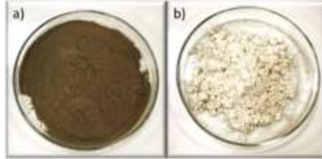
Figure 1. The Test Materials A) Alluvial Soil And B) Quick Lime
