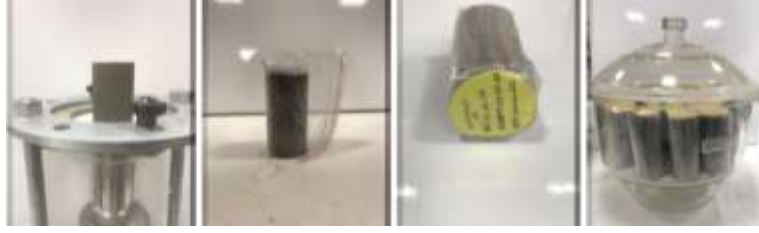
Figure 5. Sample Extruding, Sealing, Labeling and Curing Procedures
