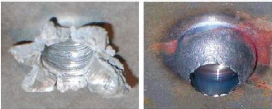
Figure 21. Friction Drilling Holes Applications a) A1382 b) AISI 1020 (Miller et al., 2006)
