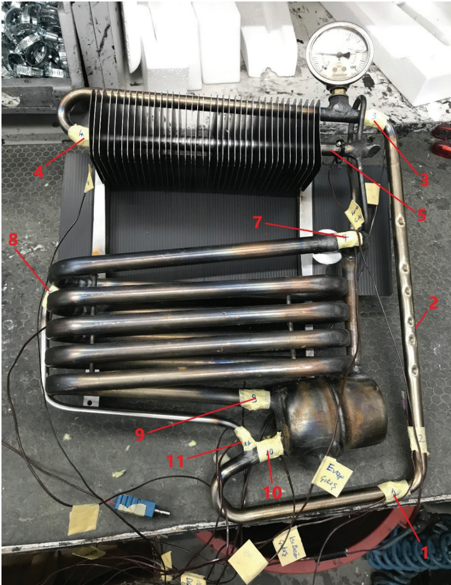
Figure 3. Temperature Measurement Points and Manometer Connection of the Absorption Cooling Device
