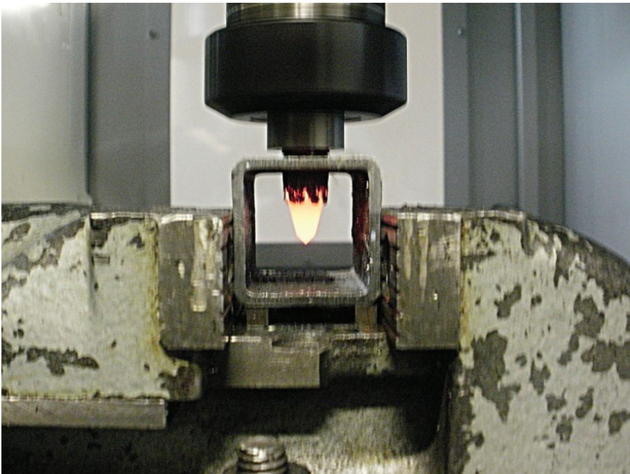
Figure 4. Friction Drilling Application to Welded Square (Doğru, 2010)
