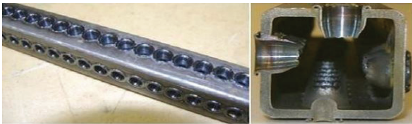
Figure 13. AISI 1015 Section Drilled with Friction Tool Perspective View b) Sectional View (Pantawane and Ahuja 2015)
