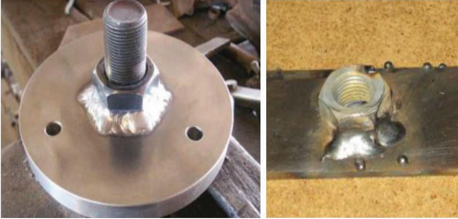
Figure 2. Nut Welding Application to the Hole Outlet (Özkan and Ünlü 2016)
